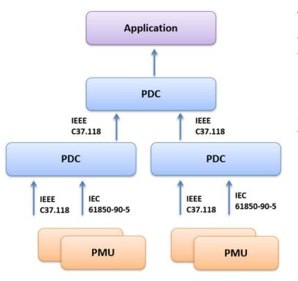
A Phasor Data Concentrator (PDC) is a function responsible for the collection, aggregation and time synchronization of data from Phasor Measurement Unit (PMU) or other PDCs and their transmission to other PDCs or to a target application.
